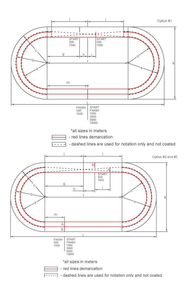
Examples of measurements of 333,33m speed skating tracks
